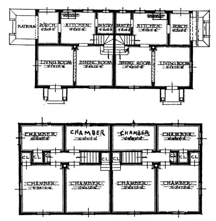
Fig. 44.—PICTURE AND PLANS OF GROUP OF POURED CONCRETE SEMI-DETACHED HOUSES IN ANTHRACITE REGION.
